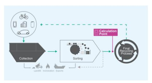
Figure 1. Recycling value chain and the point of measurement
